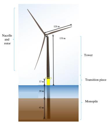
Figure 12: Main components of offshore wind turbine
